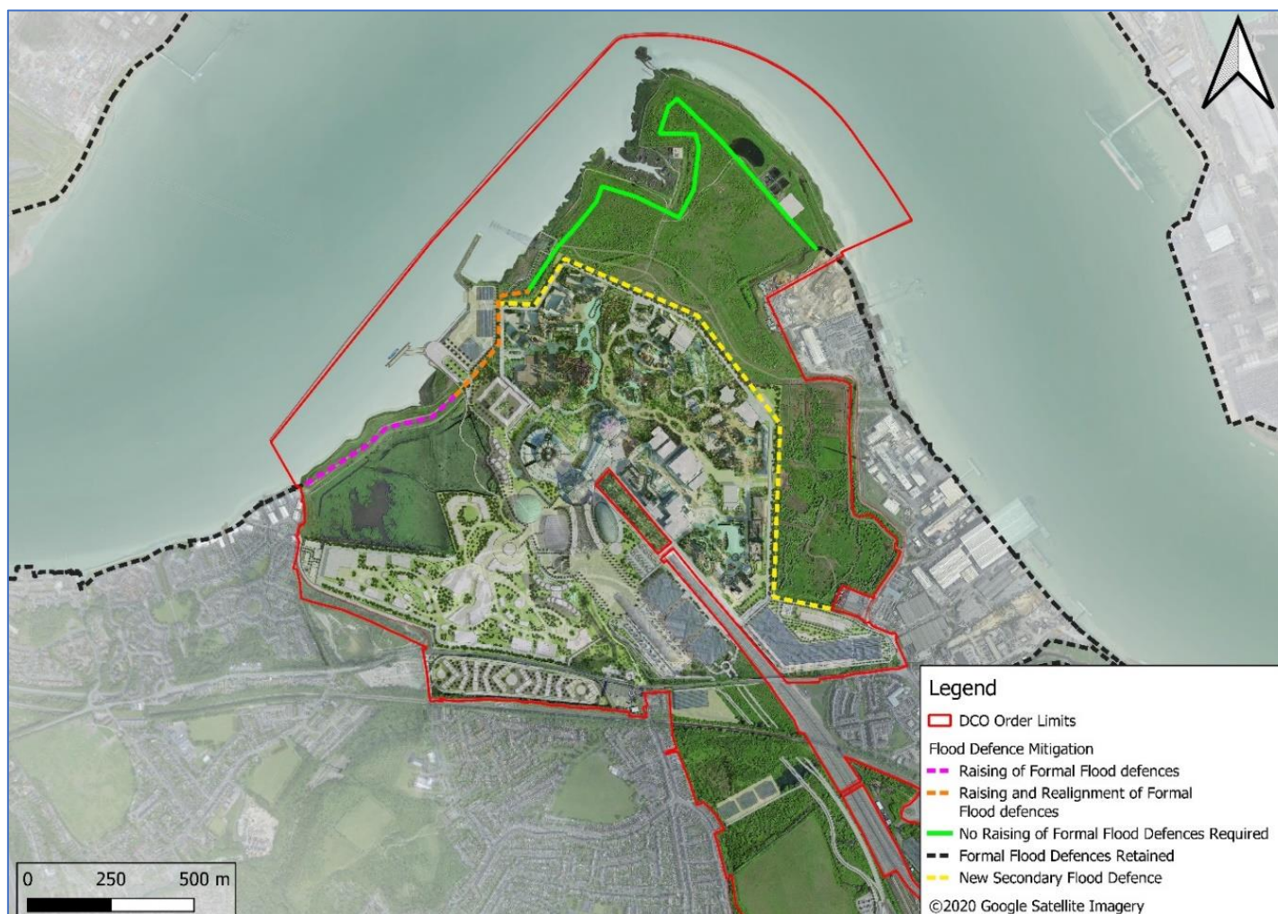
Figure 17.31: Proposed mitigation measures to provide the required standard of protection to the site from tidal overtopping.
